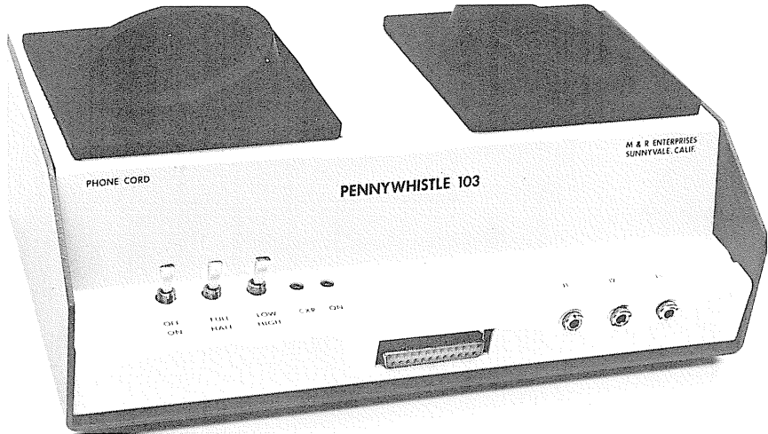
Fig. 7-20. A typical modem using an acoustical coupler.
