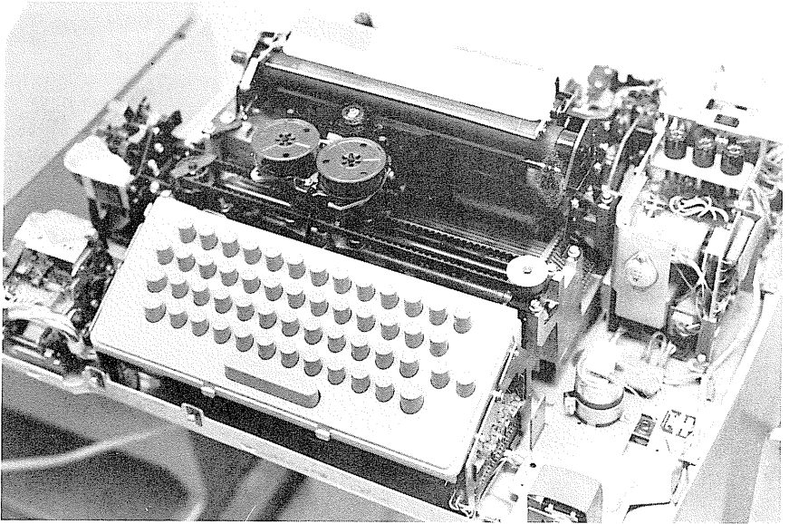
Fig. 9-3. Interior view of ASR-33 TTY.
