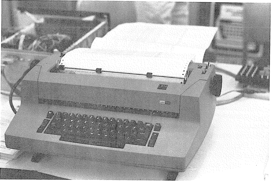
Fig. 9-4. A surplus terminal using an IBM Selectric printer mechanism.
