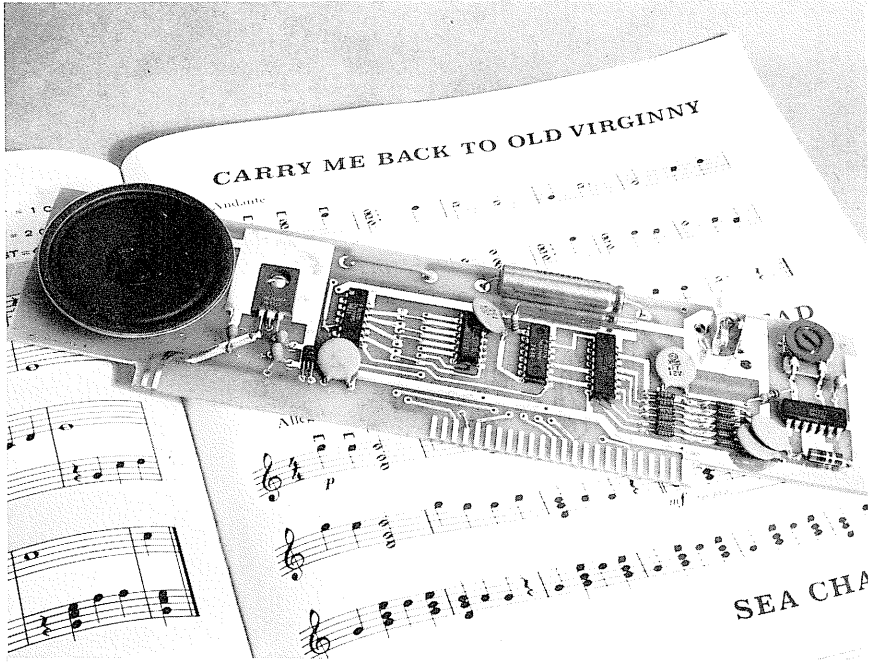
Fig. 14-2. A music synthesizer board for the S-100 bus. (Courtesy Newtech Computer Systems)
