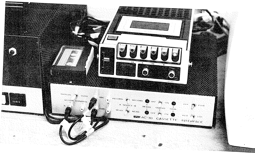
Fig. 8-6. A KC standard type tape cassette recording system.
